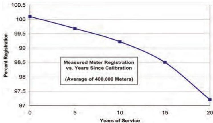
Electronic meters are a better than electromechanical meters because they do not contain moving parts in it which might get affected due to the various factors as listed above. Also they provide not only the consumed units (as is the case of electromechanical meters) but they also provide other information like the instantaneous and maximum rate of usage demands, [voltages](#), [power factor](#) and so on.
