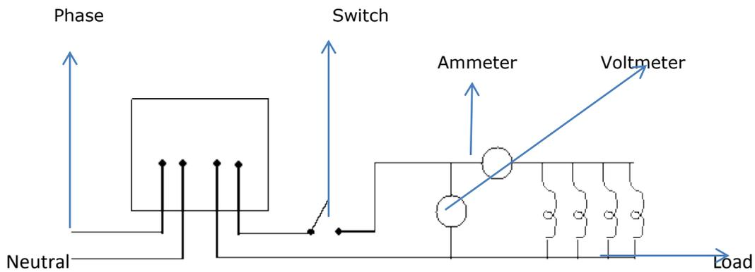
Switch of the supply through Switch 'SW' Note down the initial reading of energy meter of the switch ON note down the reading of Voltmeter and ammeter. Let the energy meter run for 10 minutes. Again note down the energy meter reading after 10 minutes. A set readings may be obtained after an interval of 5 or 10 minutes and noted in the following note
